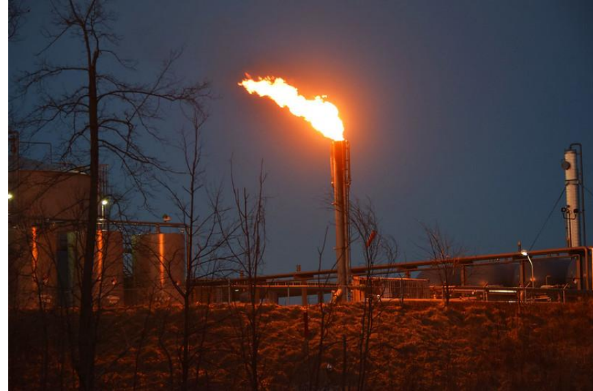
Flaring at a compressor station Photo credit: Fracktracker Alliance
